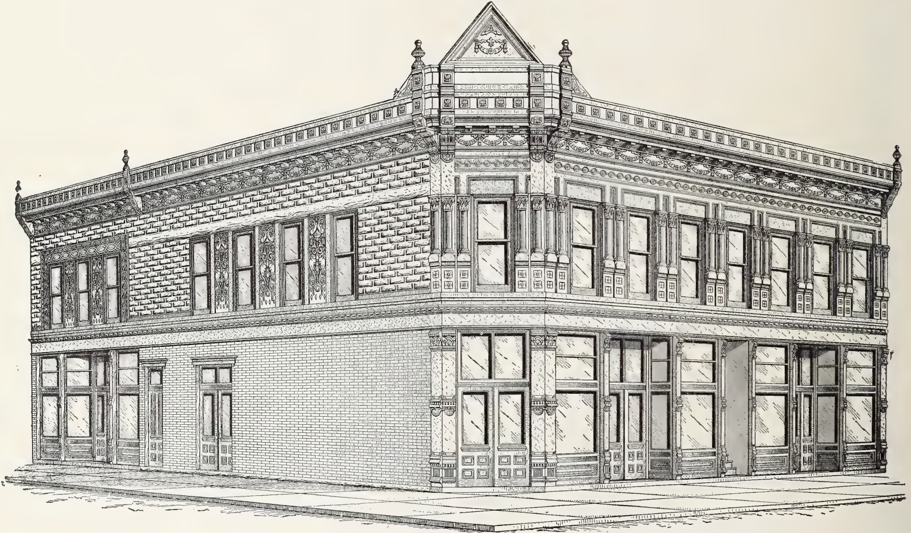
No. 1000—Illustrates a 50-foot front, with octagon cut-off corner, also showing treatment of side.
